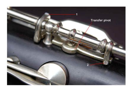
Leblanc bass speaker mechanism and close up of transfer linkage.
